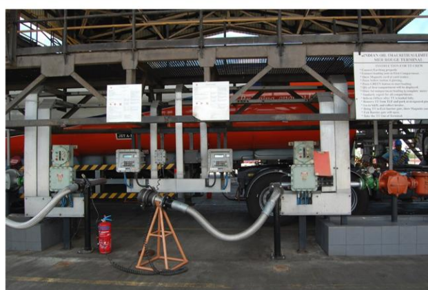
2. Verification of bulk meter carried at fuel depot using a calibrated master meter.
