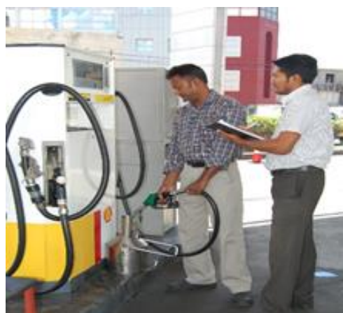
Verification of petrol pumps using calibrated checkpump measure
