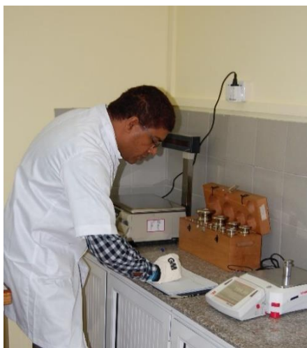
Verification of an accuracy class II electronic scale in the mass laboratory using F_2 standard
