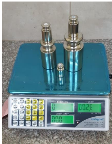
Verification of electronic scale with M_1 working standards weights
